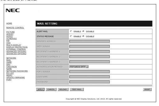
This option notifies your computer of an error message via e-mail when using wired LAN. An error message notification will be sent when an error occurs in the monitor.
