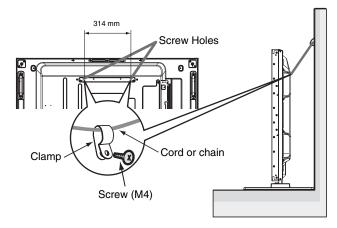
Before attaching the LCD monitor to the wall, make sure that the wall can support the weight of the monitor.
