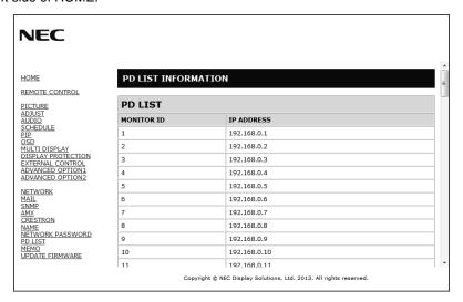
Show the list of ID and IP address of multiple monitors that are daisy-chained. Only the master monitor can show the list.
