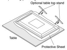
NOTE: Install the stand so the long end of the feet face forward. Use the ST-5220 for the X555UNS/X555UNV.
