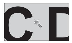
Using "SET/POINT ZOOM" button on a remote control allows to enlarge a partial of image. Press CH+/- button to zoom up or down. The image can be expanded from 1 to 10 times.
