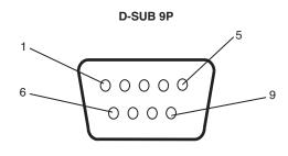
This LCD monitor uses RXD, TXD and GND lines for RS-232C control.
