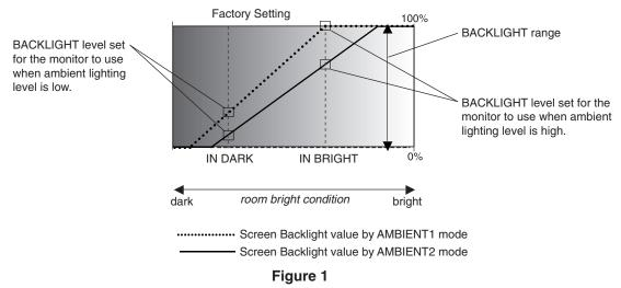
IN DARK: BACKLIGHT level set for the monitor to use when ambient lighting level is low. IN BRIGHT: BACKLIGHT level set for the monitor to use when ambient lighting level is high.
