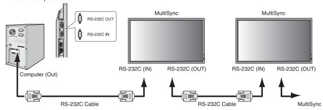
**NOTE:** If your computer is equipped only with a 25-pin serial port connector, a 25-pin serial port adapter is required. Contact your dealer for details.
