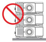
Installation example when using 3 or more projectors The following installation is recommended when installing a combination of 3 or more projectors for multi-screen projection.
