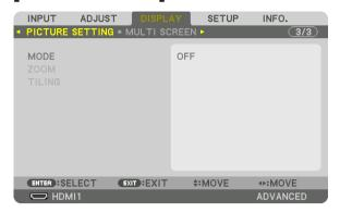
This sets the division conditions for reducing or enlarging the image area and displaying it in the desired position or for projecting using a combination of several projectors.
